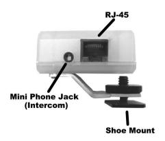
The TL-2 connects to your TLC tally controller via standard Ethernet style cable with RJ-45 connectors.
